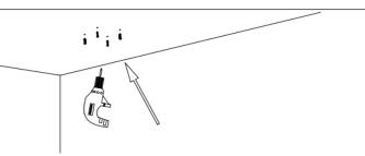
2.Use drill to drill holes ready for plastic anchors. Insert plastic anchors into hole.
