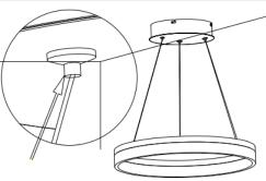
6: The length of the cable is adjustable. To determine the proper length of the fixture, hold the fixture canopy up against the outlet box in the ceiling and adjust the cable. Depress locking pin on the canopy, hold pin in place, and pull down or push up on the cable.
