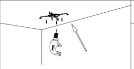
3.Attach included mounting bracket to outlet box with outlet screws. Screw anchor screws into plastic anchors to secure mounting bracket.
