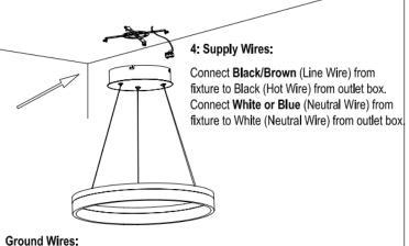
Connect **Yellow or Bare Copper** (Ground Wire) from fixture to Green (Ground Wire) from outlet box.
