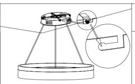
5: Attach the canopy to mounting bracket. Secure canopy with canopy screws. Twist canopy to lock fixture in place. Secure canopy with canopy screws.
