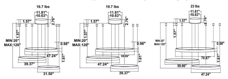
SB-S03I Remote driver, cables fixed directly to the ceiling with ring light inside. (Driver box size: L10.83" X W3.78" X H1.81")
