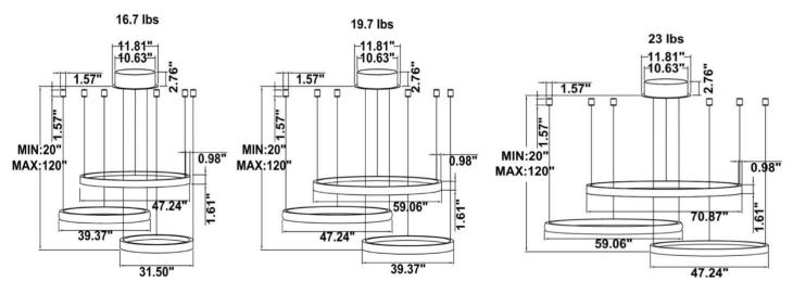
SB-S03K Remote mount with canopy, cables fixed directly to the ceiling, upper and lower light outside, center light inside.
