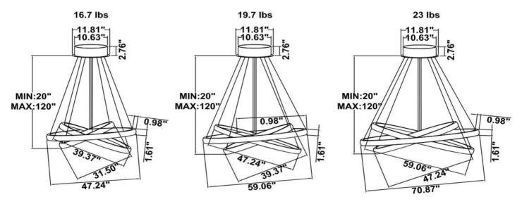
SB-S03F Canopy mount with top two ring lights outside, and the bottom ring light inside.
