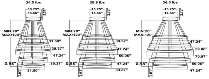
Canopy mount with first, third and last tier with inside light, second and fourth with SB-S05E outside light.
